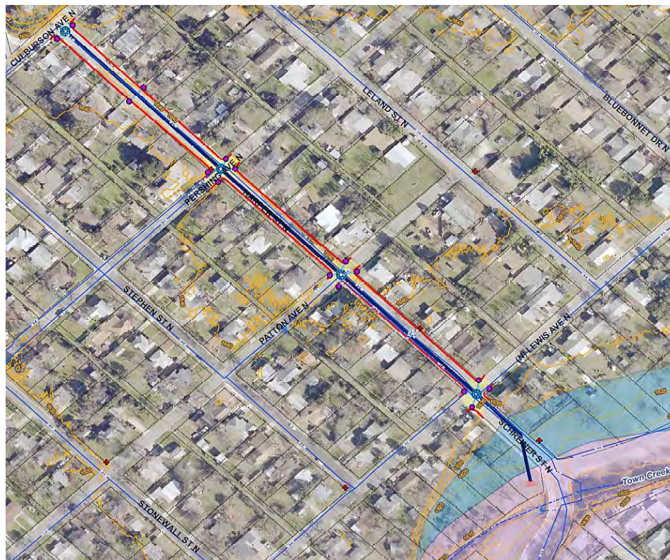
Figure 72 – Conceptual Street Drainage Improvements at Harper Street
